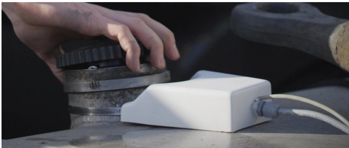
Figure 78 b.Alert Fuel installed on tank
